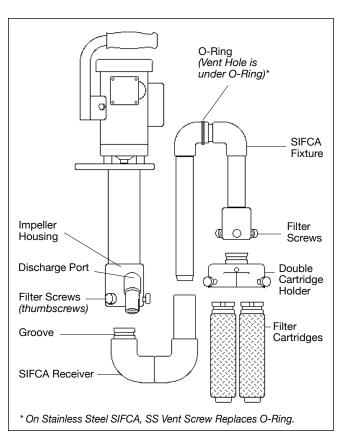
Fixture, insert into SIFCA Receiver, and push down slowly. *Note: Exposure of Vent Hole is required to bleed air from SIFCA assembly. You can feel air escaping by putting your hand over the Vent Hole while installing SIFCA Fixture.*
